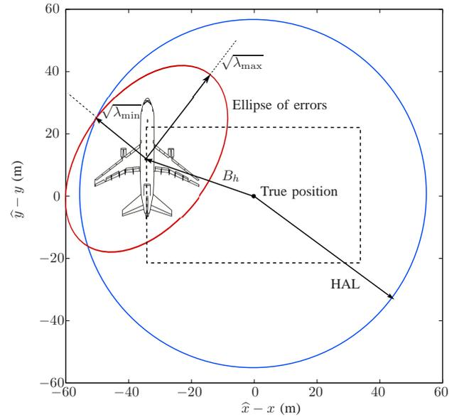
Fig. 4. The vector of systematic errors  $B_h$  and the orientation of the error ellipse. The major radius and minor radius are denoted by  $\sqrt{\lambda_{\max}}$  and  $\sqrt{\lambda_{\min}}$ , respectively.
