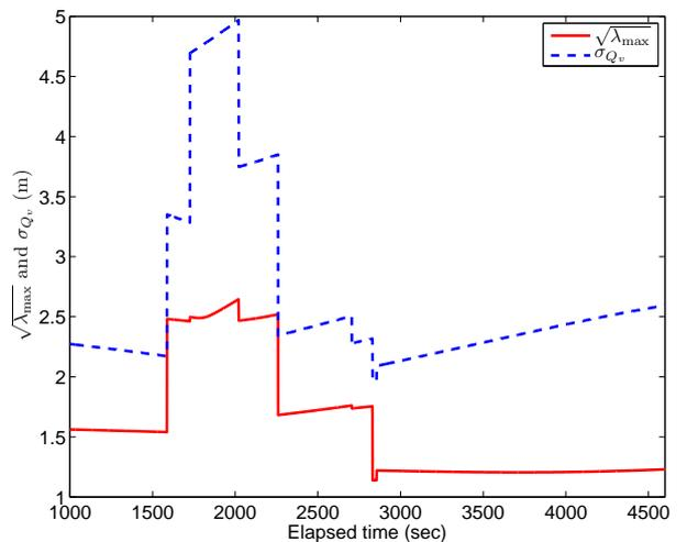
Fig. 8. The major radius of the horizontal error ellipse  $\sqrt{\lambda_{\max}}$  and the SD  $\sigma_{Q_v}$  of the vertical error  $Q_v$  as functions of the elapsed time.
