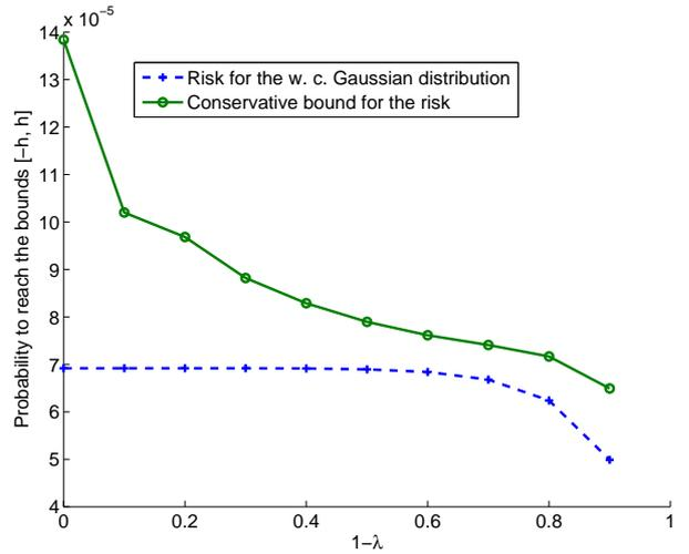
Fig. 11. The conservative bound of the vertical integrity risk per a given period of time and the vertical integrity risk calculated for the worst case (w. c.) Gaussian AR(1) process.
