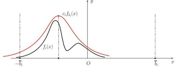
Fig. 7. Overbounding of the pseudo-range error  $\tilde{\xi}_i$  PDF by using a single Gaussian PDF with adapted mean.
