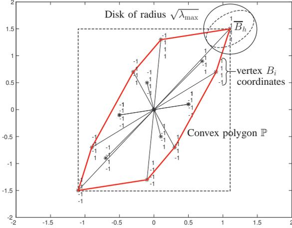
Fig. 5. The convex polygon  $\mathbb{P}$  obtained by a linear mapping (defined by the matrix  $A_h$ ) of the set  $\mathbb{B}$  onto the set  $\mathbb{P}$ .
