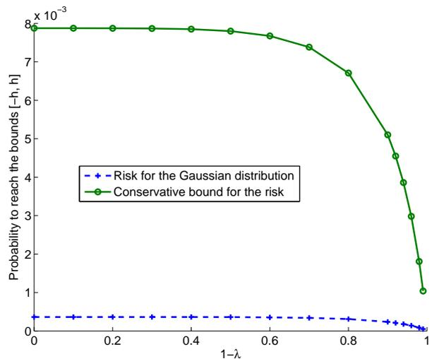
Fig. 12. The conservative bound of the vertical integrity risk per a given period of time by using the excess-mass PDF overbounding and the vertical integrity risk calculated for the Gaussian AR(1) process.
