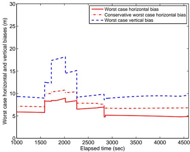
Fig. 9. The conservative worst case horizontal bias  $\|B_h^*\|_2$ , the worst case horizontal bias  $\|\bar{B}_h\|_2$  and the worst case vertical bias  $\mu$  as functions of the elapsed time.
