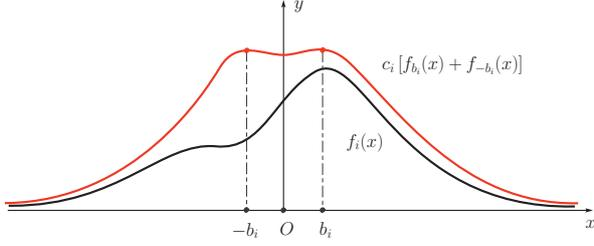
Fig. 6. Overbounding of the pseudo-range error  $\tilde{\xi}_i$  PDF by using two Gaussian PDFs.
